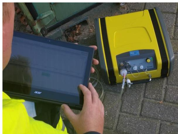
If further analysis is required, to identify unknowns or to measure even greater numbers of compounds, Gasmeter's Calcmet professional software can analyze more than 350 additional gases. The utilization of NIST reference spectra enables the analysis of over 5,000 compounds.
