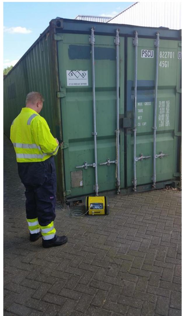
Generally, preliminary assessment is conducted with a combination of a PID detector for total VOCs; a combustible gas sensor (LEL) and a handheld electrochemical device. However, it is very important to be aware of the limitations of these instruments. For example, whilst a PID gas detector measures total VOCs, it does not provide an individual value for, say, benzene, which is a known carcinogen.
